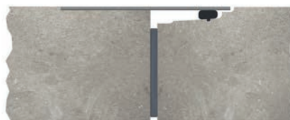
Typical flexible joints
