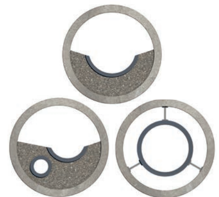
Typical reinverting and secondary lining detail
