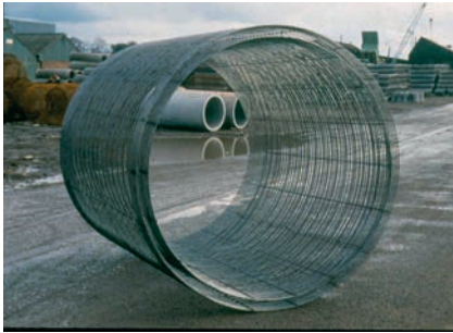
Steel cage used in concrete pipes
